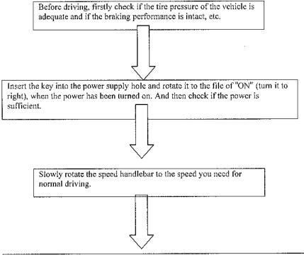
When you need parking, firstly rotate back the handlebar to decrease the speed, and then brake the tricycle, rotate the key to "OFF" and unplug the key.
