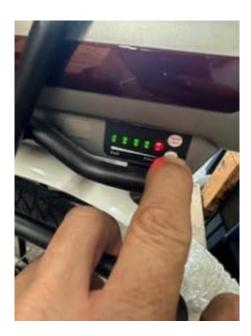
In order To turn the back light on, press the button on the side of the battery. There are multiple options; such as flash lights or steady lights etc...
